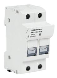
Socomec modular fuse holder, accepts Class Midget fuses, 30A, 750 VAC, 2-pole, 18-8 AWG copper only, pressure plate, 35mm DIN rail mount.
