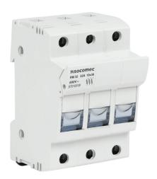
Socomec modular fuse holder, accepts Class Midget fuses, 30A, 750 VAC, 3-pole, 18-8 AWG copper only, pressure plate, 35mm DIN rail mount.
