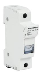
Socomec modular fuse holder, accepts Class Midget fuses, 30A, 750 VAC, 1-pole, 18-8 AWG copper only, pressure plate, 35mm DIN rail mount.
