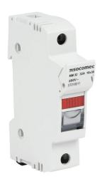
Socomec modular fuse holder, with indicator, accepts Class Midget fuses, 30A, 750 VAC, 1-pole, 18-8 AWG copper only, pressure plate, 35mm DIN rail mount. Package of 12.
