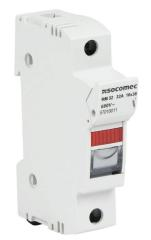
Socomec modular fuse holder, with indicator, accepts Class Midget fuses, 30A, 750 VAC, 1-pole, 18-8 AWG copper only, pressure plate, 35mm DIN rail mount.
