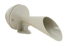
WERMA audible signal horn with trumpet, 108 dB at 1m, 100 Hz tone frequency, continuous tone(s), 115 VAC, wall mount, ABS/polycarbonate housing, off-white, IP55.
