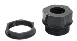
Murrplastik KDL/D-Mono series cable entry system frame, polyamide frame, TPE grommet block, M50 x 1.5mm frame, black, (1) large opening(s), UL Type 12, IP65. Package of 5. Requires (1) Murrplastik KDT/X series large grommets.
