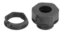
Murrplastik KDL/D-Mono series cable entry system frame, polyamide frame, M32 x 1.5mm, black, (1) medium opening(s), IP65. Package of 5. Requires (1) Murrplastik KDT/X series medium grommets.
