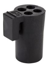
Murrplastik KDT/X series small grommet, 4 opening(s), TPE, black, accepts 4mm diameter cable. Package of 4. For use with Murrplastik KDL/D series cable entry system frame.
