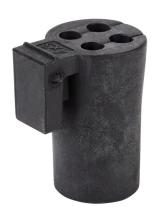
Murrplastik KDT/X series general purpose grommet, 4 opening(s), TPE, small, black, accepts 3mm diameter cable, IP65. Package of 4. For use with Murrplastik KDL/D series cable entry system frame.
