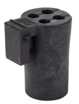
Murrplastik KDT/X series small grommet, 4 opening(s), TPE, black, accepts 3mm diameter cable. Package of 4. For use with Murrplastik KDL/D series cable entry system frame.
