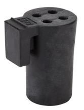
Murrplastik KDT/X series small grommet, 4 opening(s), TPE, black, accepts 2mm diameter cable. Package of 4. For use with Murrplastik KDL/D series cable entry system frame.
