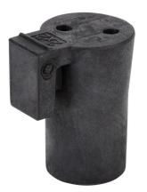
Murrplastik KDT/X series small grommet, 2 opening(s), TPE, black, accepts 2mm diameter cable. Package of 4. For use with Murrplastik KDL/D series cable entry system frame.
