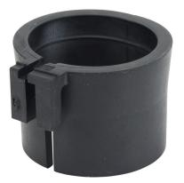
Murrplastik KDT/X series large grommet, 1 opening(s), TPE, black, accepts 29-30mm diameter cable, UL Type 12. Package of 4. For use with Murrplastik KDL/D series cable entry system frame.
