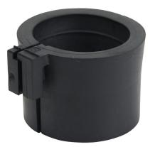
Murrplastik KDT/X series large grommet, 1 opening(s), TPE, black, accepts 27-28mm diameter cable, UL Type 12. Package of 4. For use with Murrplastik KDL/D series cable entry system frame.
