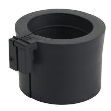
Murrplastik KDT/X series large grommet, 1 opening(s), TPE, black, accepts 26-27mm diameter cable, UL Type 12. Package of 4. For use with Murrplastik KDL/D series cable entry system frame.
