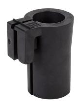
Murrplastik KDT/X series general purpose grommet, 1 opening(s), TPE, small, black, accepts 10 to 11mm diameter cable, IP65. Package of 4. For use with Murrplastik KDL/D series cable entry system frame.
