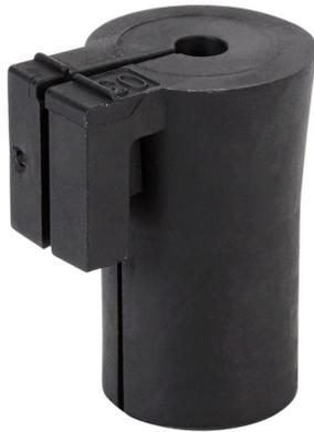
Murrplastik KDT/X series small grommet, 1 opening(s), TPE, black, accepts 3-4mm diameter cable. Package of 4. For use with Murrplastik KDL/D series cable entry system frame.
