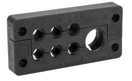
Murrplastik KDL/D series cable entry system frame, polypropylene frame, TPE grommet block, 16-pin frame, black, (6) small and (1) medium opening(s), UL Type 1, 12 and 4X indoor use only, IP65.
