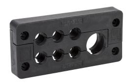
Murrplastik KDL/D series cable entry system frame, polypropylene frame, TPE grommet block, 16mm, black, (6) small and (1) medium opening(s), IP65. Requires (6) Murrplastik KDT/X series small grommets and (1) medium grommet.
