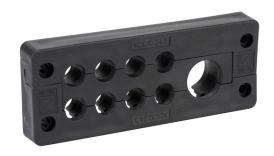
Murrplastik KDL/D series cable entry system frame, polypropylene frame, TPE grommet block, 24-pin frame, black, (8) small and (1) medium opening(s), UL Type 1, 12 and 4X indoor use only, IP65.
