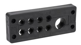
Murrplastik KDL/D series cable entry system frame, polypropylene frame, TPE grommet block, 24mm, black, (8) small and (1) medium opening(s), IP65. Requires (8) Murrplastik KDT/X series small grommets and (1) medium grommet.
