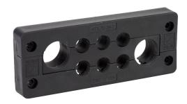
Murrplastik KDL/D series cable entry system frame, polypropylene frame, TPE grommet block, 24mm, black, (6) small and (2) medium opening(s), IP65. Requires (6) Murrplastik KDT/X series small grommets and (2) medium grommets.
