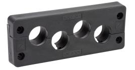
Murrplastik KDL/D series cable entry system frame, polypropylene frame, TPE grommet block, 24-pin frame, black, (4) medium opening(s), UL Type 1, 12 and 4X indoor use only, IP65. Requires (4) Murrplastik KDT/X series medium grommets.
