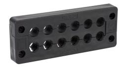
Murrplastik KDL/D series cable entry system frame, polypropylene frame, TPE grommet block, 24-pin frame, black, (12) small opening(s), UL Type 1 and 12, IP65. Requires (12) Murrplastik KDT/X series small grommets.
