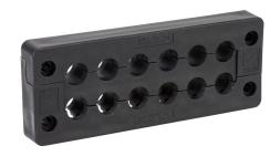
Murrplastik KDL/D series cable entry system frame, polypropylene frame, TPE grommet block, 24mm, black, (12) small opening(s), IP65. Requires (12) Murrplastik KDT/X series small grommets.
