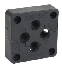
Murrplastik KDL/D-R series cable entry system frame, polypropylene frame, TPE grommet block, 50mm diameter frame, black, (4) small opening(s), UL Type 12, IP65. Requires (4) Murrplastik KDT/X series small grommets.
