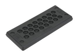
Murrplastik KDP/Z series cable entry system frame, polypropylene frame, TPS grommet block, 24-pin frame, black, (23) 5-9mm opening(s), UL Type 4X and 12, IP65 IP66 IP67. Package of 5.
