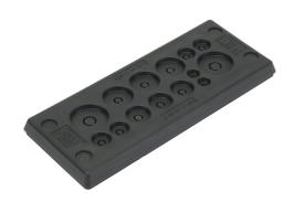
Murrplastik KDP/Z series cable entry system frame, polypropylene frame, TPS grommet block, 24-pin frame, black, (2) 3-6mm, (4) 5-9mm, (3) 7.5-12mm, (3) 10-16mm and (2) 14-20mm opening(s), UL Type 4X and 12, IP65 IP66 IP67. Package of 5.
