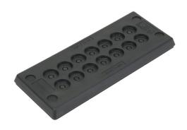
Murrplastik KDP/Z series cable entry system frame, polypropylene frame, TPS grommet block, 24-pin frame, black, (14) 7.5-12mm opening(s), UL Type 4X and 12, IP65 IP66 IP67. Package of 5.
