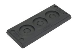
Murrplastik KDP/Z series cable entry system frame, polypropylene frame, TPS grommet block, 24-pin frame, black, (3) 22-33mm opening(s), UL Type 4X and 12, IP65 IP66 IP67. Package of 5.
