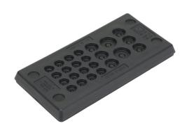
Murrplastik KDP/Z series cable entry system frame, polypropylene frame, TPS grommet block, 16-pin frame, black, (16) 3-6mm, (6) 5-9mm and (2) 7.5-12mm opening(s), UL Type 4X and 12, IP65 IP66 IP67. Package of 5.
