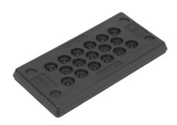
Murrplastik KDP/Z series cable entry system frame, polypropylene frame, TPS grommet block, 16-pin frame, black, (17) 5-9mm opening(s), UL Type 4X and 12, IP65 IP66 IP67. Package of 5.
