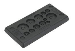
Murrplastik KDP/Z series cable entry system frame, polypropylene frame, TPS grommet block, 16-pin frame, black, (2) 3-5mm, (4) 5-9mm, (2) 7.5-12mm, (2) 10-16mm and (2) 14-20mm opening(s), UL Type 4X and 12, IP65 IP66 IP67. Package of 5.
