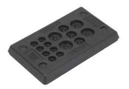
Murrplastik KDP/Z series cable entry system frame, polypropylene frame, TPS grommet block, 10-pin frame, black, (8) 3-8mm, (3) 5-9mm and (4) 7.5-12mm opening(s), UL Type 4X and 12, IP65 IP66 IP67. Package of 5.
