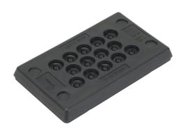
Murrplastik KDP/Z series cable entry system frame, polypropylene frame, TPS grommet block, 10-pin frame, black, (14) 5-9mm opening(s), UL Type 4X and 12, IP65 IP66 IP67. Package of 5.
