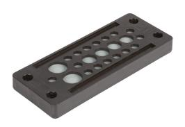
Murrplastik KDP/X series cable entry system frame, polyamide frame, 24-pin frame, black, (16) 3.5-6.5mm, (4) 7.5-11.5mm and (2) 9-14mm opening(s), UL Type 12 and 1, IP65.
