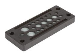
Murrplastik KDP/X series cable entry system frame, polyamide frame, 24mm, black, (16) 3.5-6.5mm, (4) 7.5-11.5mm and (2) 9-14mm opening(s), IP65.
