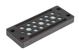
Murrplastik KDP/X series cable entry system frame, polyamide frame, 24mm, black, (2) 3.5-6.5mm, (14) 5-9.2mm and (3) 7.5-11.5mm opening(s), IP65.
