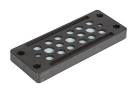
Murrplastik KDP/X series cable entry system frame, polyamide frame, 24-pin frame, black, (2) 3.5-6.5mm, (14) 5-9.2mm and (3) 7.5-11.5mm opening(s), UL Type 12 and 1, IP65.
