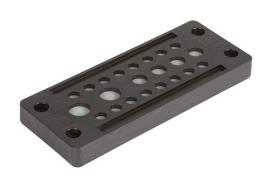
Murrplastik KDP/X series cable entry system frame, polyamide frame, 24mm, black, (16) 3-6.5mm, (4) 5-9.2mm and (2) 8-12.5mm opening(s), IP65.
