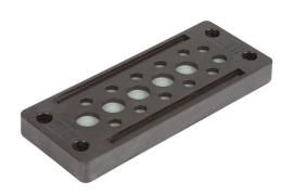
Murrplastik KDP/X series cable entry system frame, polyamide frame, 24-pin frame, black, (11) 3-6.5mm, (1) 4.1-8.1mm and (5) 8-12.5mm opening(s), UL Type 12 and 1, IP65.
