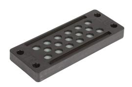
Murrplastik KDP/X series cable entry system frame, polyamide frame, 24mm, black, (17) 5-9.2mm opening(s), IP65.
