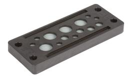
Murrplastik KDP/X series cable entry system frame, polyamide frame, 24-pin frame, black, (6) 3-6.5mm, (4) 5-9.2mm and (4) 9.6-15.9mm opening(s), UL Type 12 and 1, IP65.
