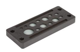
Murrplastik KDP/X series cable entry system frame, polyamide frame, 24-pin frame, black, (2) 3-5.5mm, (6) 4.1-8.1mm, (4) 9-14mm and (1) 14-20mm opening(s), UL Type 12 and 1, IP65.
