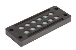
Murrplastik KDP/X series cable entry system frame, polyamide frame, 24-pin frame, black, (12) 8-12mm opening(s), UL Type 12 and 1, IP65.
