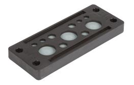
Murrplastik KDP/X series cable entry system frame, polyamide frame, 24-pin frame, black, (4) 3-6.5mm, (4) 5-9.2mm and (3) 14-20mm opening(s), UL Type 12 and 1, IP65.
