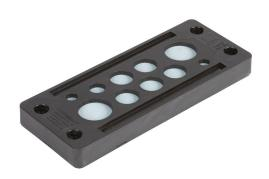
Murrplastik KDP/X series cable entry system frame, polyamide frame, 24-pin frame, black, (2) 3-6.5mm, (1) 5-9.2mm, (5) 9-14mm and (2) 14-20mm opening(s), UL Type 12 and 1, IP65.
