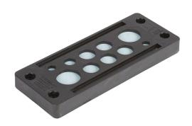
Murrplastik KDP/X series cable entry system frame, polyamide frame, 24mm, black, (2) 3-6.5mm, (1) 5-9.2mm, (5) 9-14mm and (2) 14-20mm opening(s), IP65.
