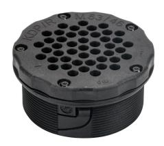
Murrplastik KDP/R series general purpose cable entry system frame, polyamide frame, M63 x 1.5mm frame, black, (46) 1.5-3.1mm opening(s), IP65.
