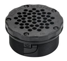
Murrplastik KDP/R series cable entry system frame, polyamide frame, M63 x 1.5mm frame, black, (46) 1.5-3.1mm opening(s), UL Type 1, IP65.
