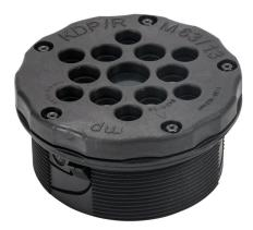
Murrplastik KDP/R series general purpose cable entry system frame, polyamide frame, M63 x 1.5mm frame, black, (6) 3-5.5mm, (6) 3.5-6.5mm and (1) 6-10mm opening(s), IP65.
