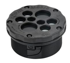
Murrplastik KDP/R series general purpose cable entry system frame, polyamide frame, M63 x 1.5mm frame, black, (2) 3-6.5mm, (4) 5-9.2mm and (2) 9.6-15.9mm opening(s), IP65.
