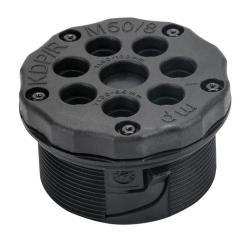
Murrplastik KDP/R series general purpose cable entry system frame, polyamide frame, M50 x 1.5mm frame, black, (7) 3.5-6.5mm and (1) 6-10mm opening(s), IP65.
