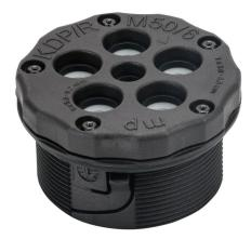
Murrplastik KDP/R series cable entry system frame, polyamide frame, M50 x 1.5mm frame, black, (1) 3-5.5mm and (5) 5-9.2mm opening(s), UL Type 1, IP65.
