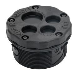
Murrplastik KDP/R series cable entry system frame, polyamide frame, M50 x 1.5mm frame, black, (3) 6-10mm and (1) 9.6-15.9mm opening(s), UL Type 1, IP65.
