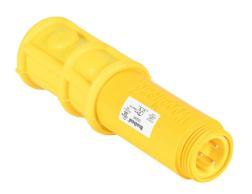
Molex pendant switch, silicone rubber/PVC, single pushbutton, flush, yellow, snap action, (1) N.O. contact(s), 7/8in - 16 UN2 3-pin male. Requires 7/8in - 16 UN2 3-pin connection cable.
