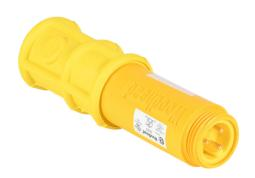
Molex pendant switch, nitrile rubber/PVC, single pushbutton, flush, yellow, snap action, (1) N.O./(1) N.C. contact(s), 7/8in - 16 UN2 3-pin male. Requires 7/8in - 16 UN2 3-pin connection cable.
